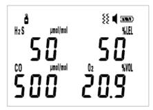
The screen will display calibrating concentration, after you input the standard gas, the BX616 detector will start to analyze.
